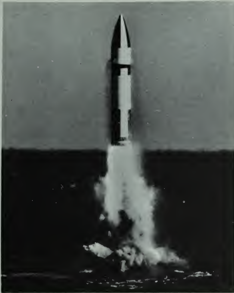
A Polaris 2,500 mile range A-3 missile fired from USS Lewis and Clark (SSBN-644)
